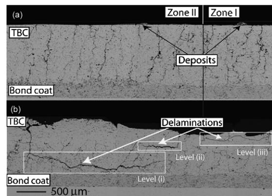
Fig. 2. Micrographs of cross-sections through the TBC along the plane marked in Fig. 1: (a) SE images of zones I and II. Note the dense vertical cracks (DVC) with spacing,  $d = 0.2$  mm, and the deposits on the surface. (b) SE image of zone III close to the spalled region. Delaminations at three different levels are apparent. In each case the delaminations originate from channel cracks with separation,  $s \sim 1$  mm (see Fig. 3 for details on channel crack morphology).
