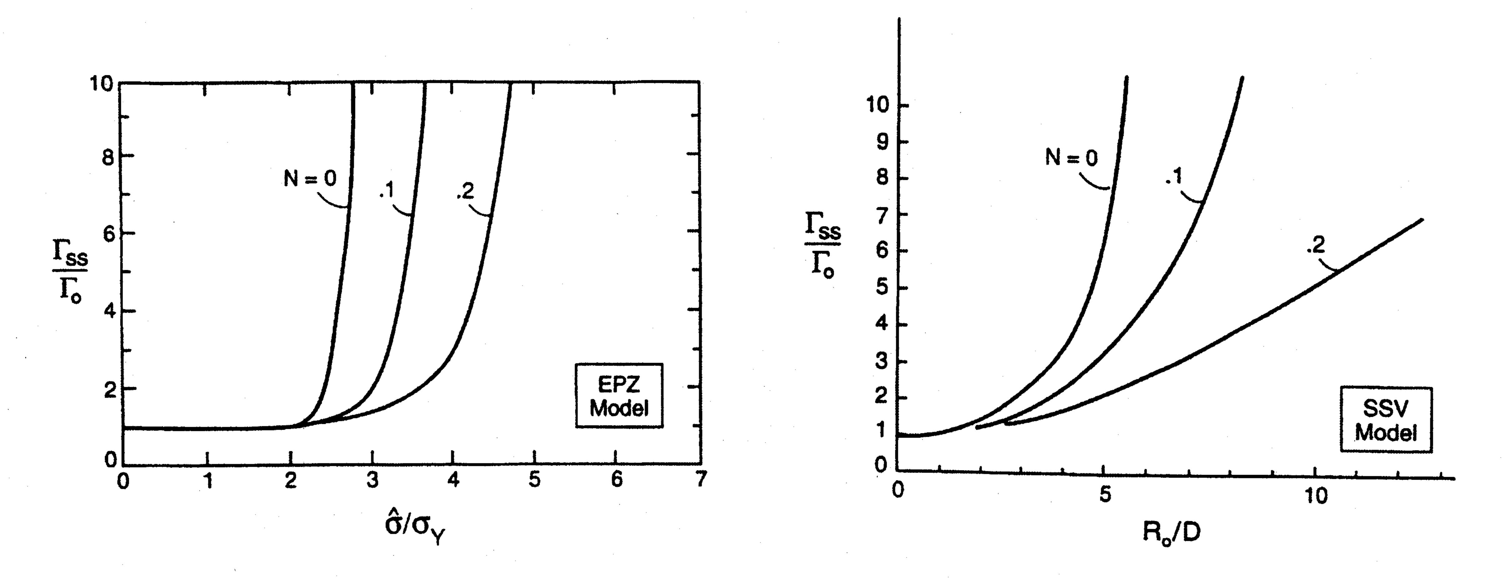
Figure 3. The ratio of steady-state macroscopic work of fracture to work of separation  $\Gamma_{ss}/\Gamma_0$ , for the EPZ and SSV models specialized to mode I growth in a homogeneous elastic-plastic solid. The EPZ results are from Tvergaard and Hutchinson (1992) with  $\nu = 0.3$ ,  $\lambda_1 = 0.15$  and  $\lambda_2 = 0.5$ . The SSV results are from Suo et al. (1993) with  $\nu = 0.3$ .
