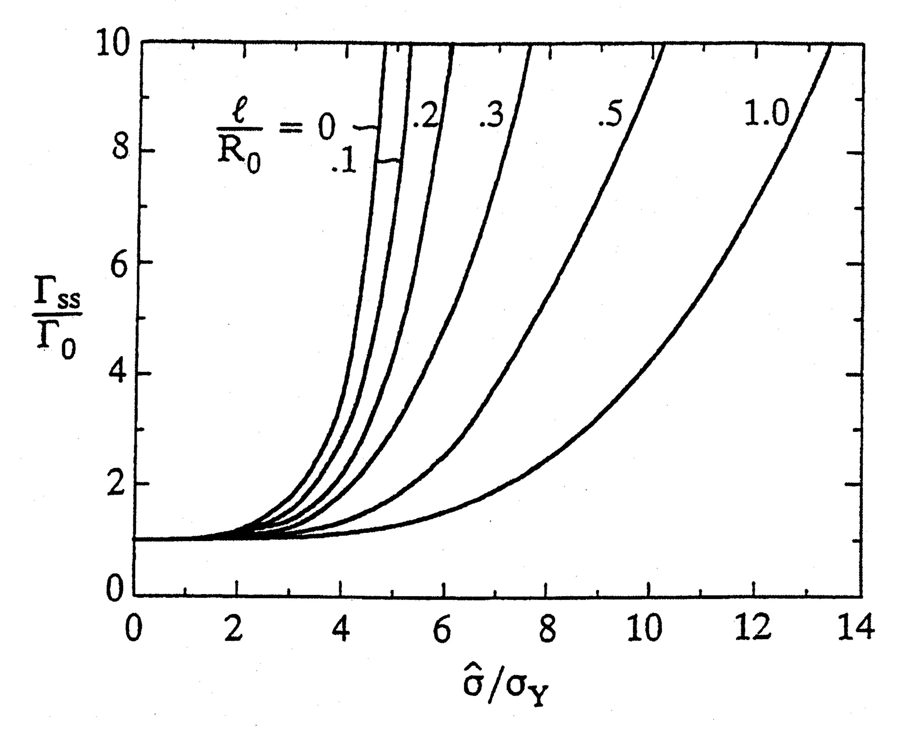
Figure 7. The influence of strain gradient hardening on  $\Gamma_{ss}/\Gamma_0$  as predicted by the EPZ model for mode I growth in a homogeneous elastic-plastic solid characterized by  $J_2$  SGP theory. The limit  $\ell/R_0=0$  corresponds to conventional  $J_2$  flow theory (Figure 3). The results are taken from Wei and Hutchinson (1997) and were computed with N=0.2,  $\nu=0.3$ ,  $\lambda_1=0.15$  and  $\lambda_2=0.5$ .
