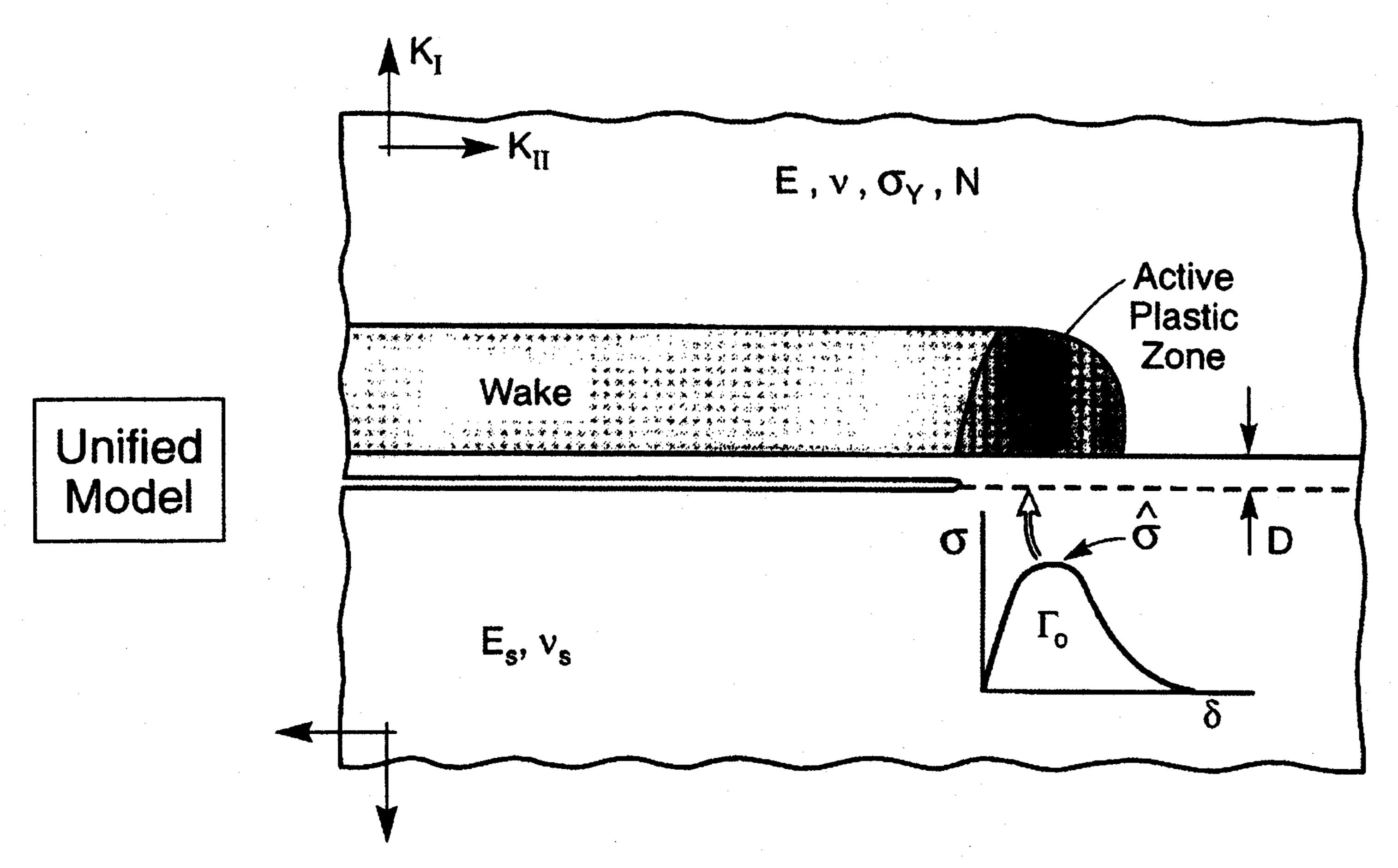
Figure 4. The unified model for crack growth along a bi-material interface under small scale yielding. The model incorporates the plasticity-free strip from the SSV model and the embedded traction-separation characterization of the interface from the EPZ model.
