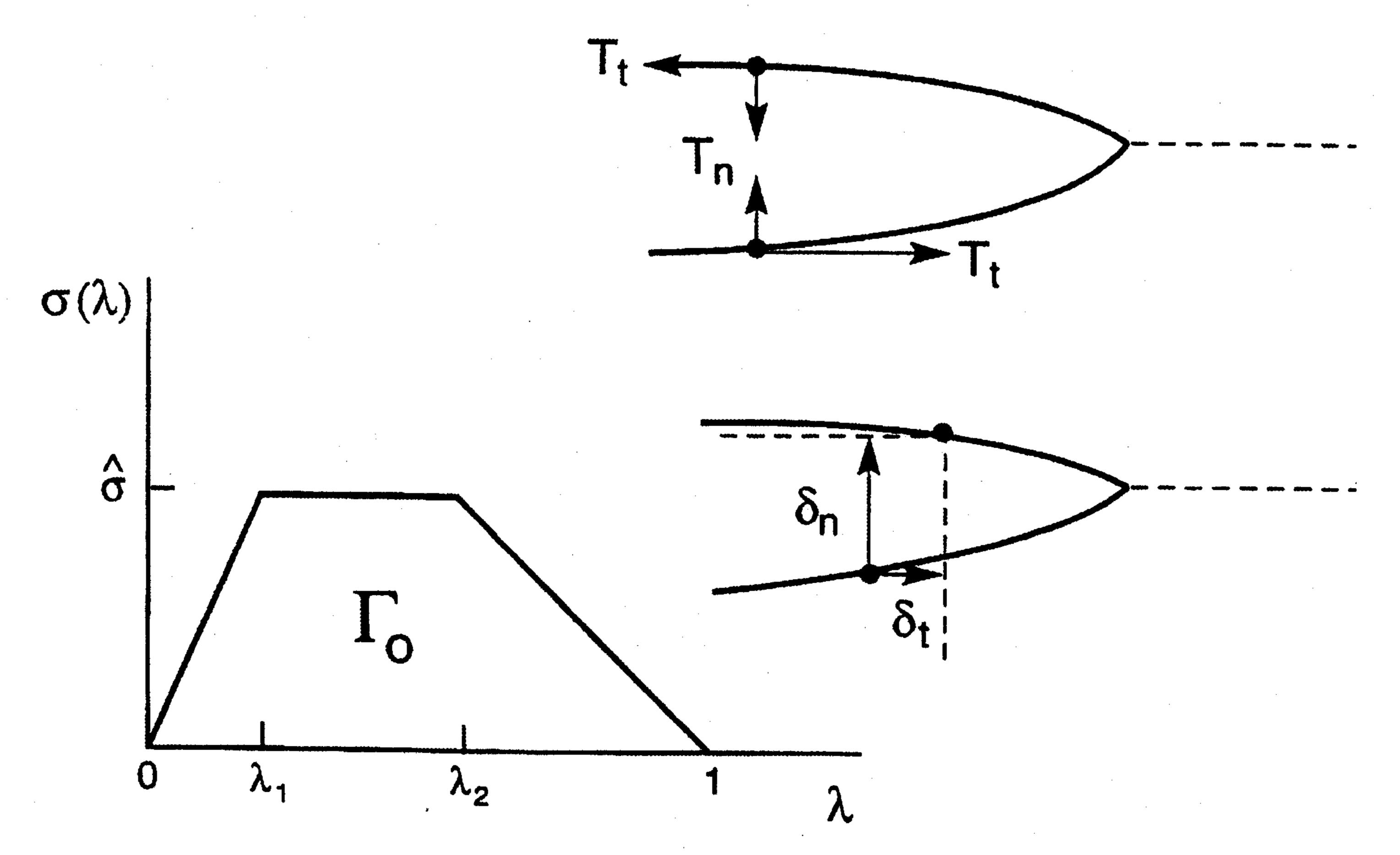
Figure 2. The traction-separation behavior characterizing the interface in the EPZ model and the unified model.
