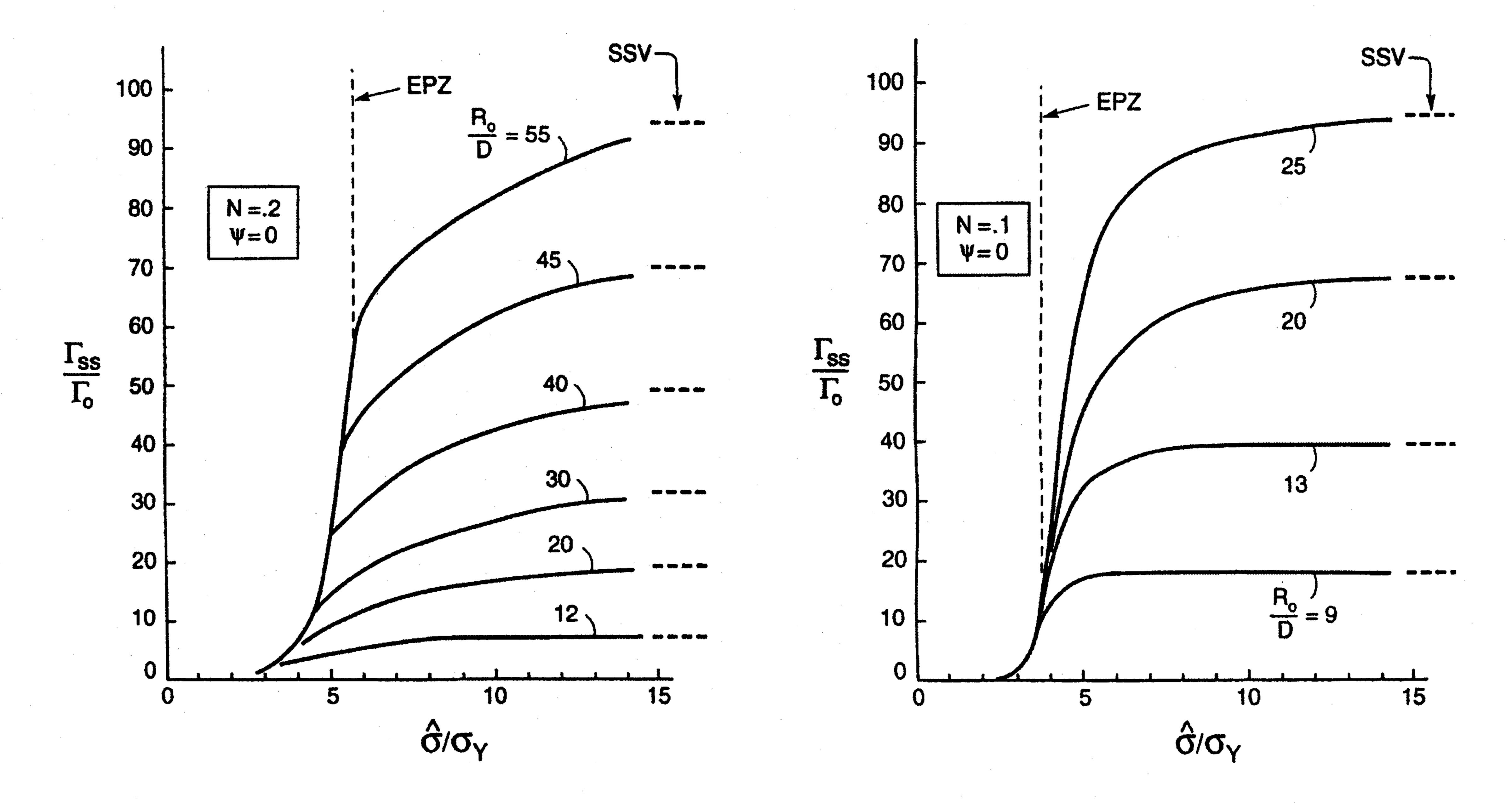
Figure 5. The ratio of the macroscopic work of fracture to work of separation,  $\Gamma_{ss}/\Gamma_0$ , for the unified model for mode I ( $\psi = 0$ ) steady-state crack growth along a bi-material interface joining an elastic-plastic solid to a rigid solid. The parameters used in carrying out the calculations are  $\nu = 0.3$ ,  $\lambda_1 = 0.15$ ,  $\lambda_2 = 0.5$  and  $\delta_n^c/\delta_t^c = 1$ .
