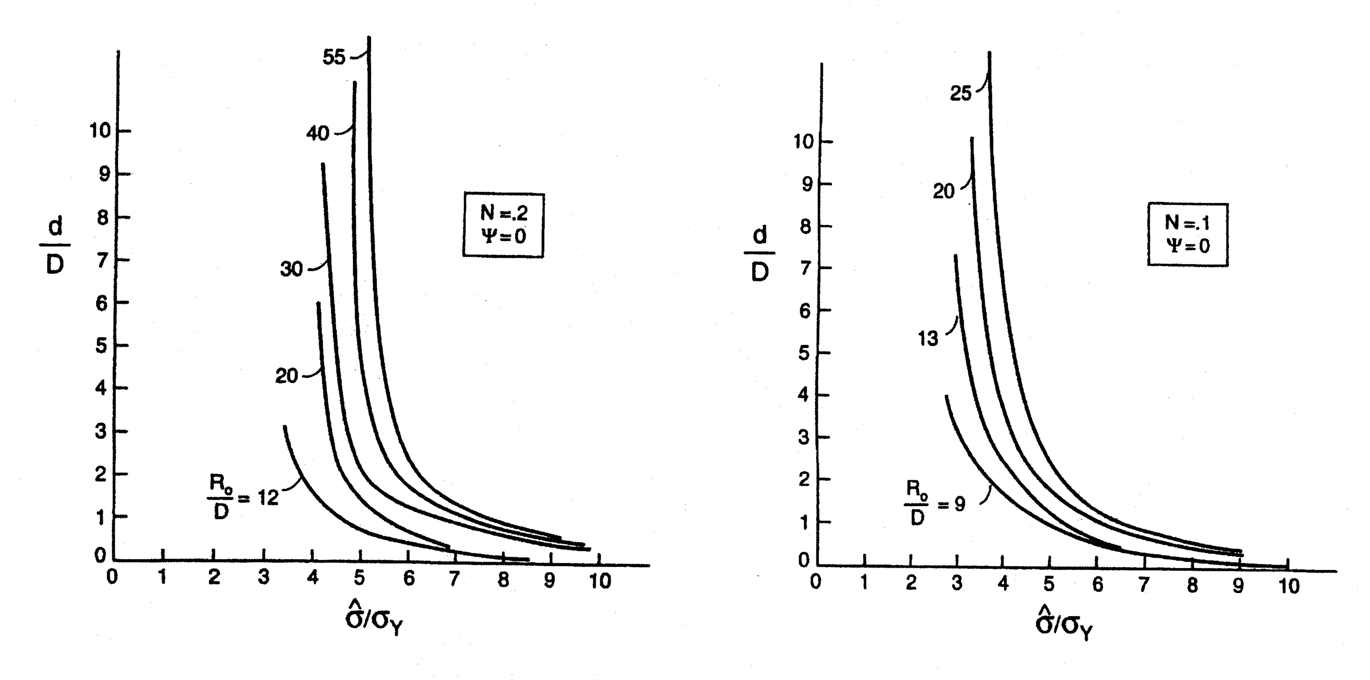
Figure 6. The ratio of the length of the separation zone at the interface to the thickness of the plasticity-free strip d/D, for the examples of Figure 5.
