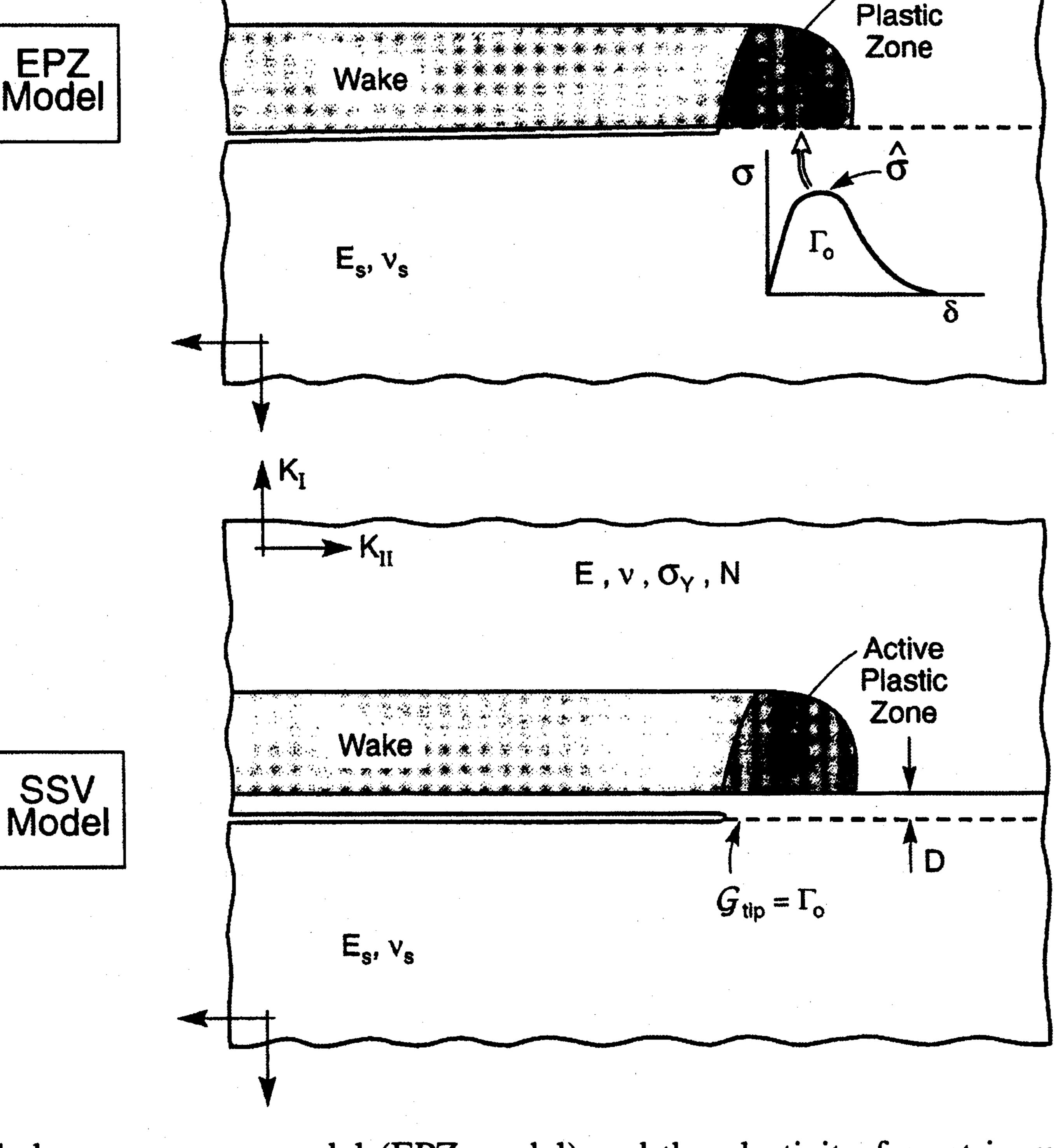
Figure 1. The embedded process zone model (EPZ model) and the plasticity-free strip model (SSV model) for a bi-material interface where the upper material is elastic-plastic and the lower material is elastic. The study is limited to steady-state crack growth in small scale yielding wherein the active plastic zone is small compared to the crack length. The finite length crack is replaced by a semi-infinite crack loaded remotely by the elastic K-field.
