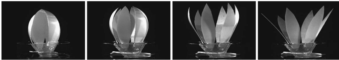
Figure 5. A floral mimic made of paper–plastic bilayer petals shows a controllable blooming and wilting response. When dipped in water, the petals open and the flower blooms, while when the water supply is exhausted, the bilayer dries out and the flower closes (see electronic supplementary material, movies S6 and S7). The length of the petals is about 4 cm, and the typical time scale of a cycle is an hour.
