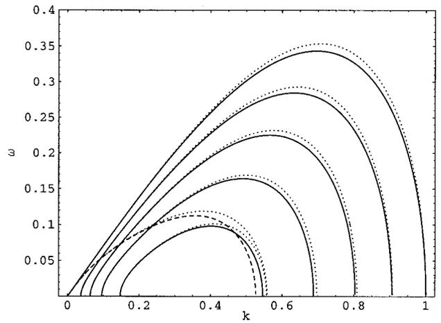
FIG. 5. Comparison of Saville's (Ref. 33) dispersion relation for a zero viscosity fluid as a function of field strength, for  $\beta=77$ . The solid lines are Saville's results for infinite conductivity, with field strengths,  $\Omega_0^2 = 0, 0.97, 1.93, 2.90, 3.8$  from the uppermost to the lowermost, respectively. The dashed line is for zero conductivity and  $\Omega_0^2 = 4.83$ . The dotted lines are from Eq. (19).
