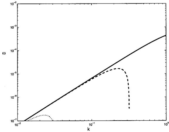
FIG. 17. The dependence of the growth rate on viscosity for  $E_\infty = 1$  kV/cm,  $K = 0.01$   $\mu$ S/cm,  $\beta = 80$ ,  $r_0 = 0.05$  cm, and  $\gamma/\rho = 73$ . The uppermost solid curve shows the dispersion relation for an inviscid fluid, the middle curve has  $\mu = 0.01$  P, and the lowermost curve has  $\mu = 1$  P. Even a very small viscosity shifts the most unstable wavelength into the  $k < 1$  long wavelength regime, and greatly suppresses the growth rate.
