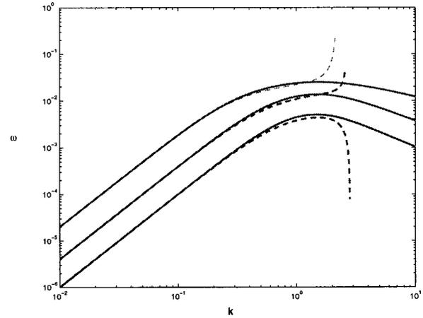
FIG. 16. Comparison of our inviscid whipping mode formula (dashed) with Saville’s exact formula (solid) for  $K^*=0.7$  and for field strengths  $\Omega_0 = 2.2, 4.4, 9.8$ . (The maximum growth rate increases with the field strength.) Our asymptotic formula deviates from Saville’s when  $k \approx 1$ , because the approximations underlying it break down.
