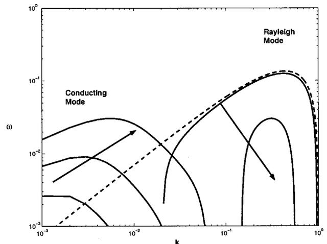
FIG. 7. Field dependence of the instability growth rate  $\omega$  for a fluid with  $\nu = 140$  cP,  $\gamma = 65$  dyn/cm, conductivity  $K = 5.8\mu$  and  $\epsilon = 78$ . As the field is increased (direction indicated by arrows) the “Rayleigh mode” is suppressed and the conducting mode becomes dominant.
