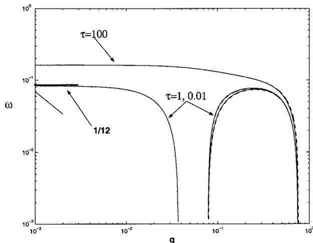
FIG. 6. Comparison of Saville’s (Ref. 34) dispersion relation for an infinite viscosity fluid with different finite electrical relaxation time  $\tau = \epsilon/K\gamma/(\mu r_0) = 0.01, 1, \text{ and } 100$ , respectively. The rightmost lines show nonoscillatory modes (i.e.,  $\text{Im } \omega = 0$ ) and the leftmost lines show oscillatory modes. The result from the dispersion relation [Eq. (19)] (dashed lines) is superimposed on Saville’s solution (solid lines) with no discernible difference.
