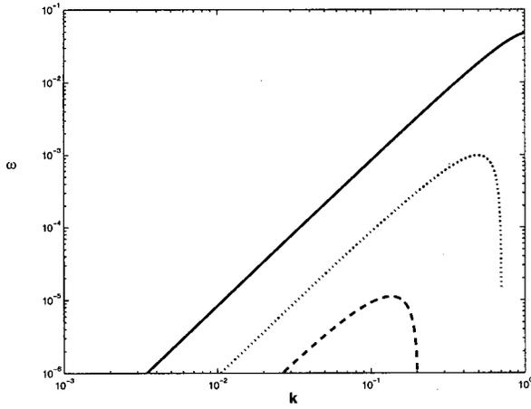
FIG. 18. The dependence of the growth rate on surface charge for a  $r_0 = 100 \mu\text{m}$  water jet ( $K=0.01 \mu\text{S/cm}$ ,  $\beta=80$ ,  $\nu=0.01$ ) in an electric field  $E_\infty=1 \text{ kV/cm}$ . The lowermost solid curve shows the dispersion relation for an uncharged fluid, the middle curve has  $\sigma_0=0.01$  and the solid curve has  $\sigma_0=0.1$ .
