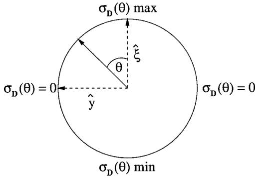
FIG. 15. Picture of the cross section of a jet.  $\hat{\mathbf{t}}$  points out of the plane of the page. The asymmetric part of the surface charge density,  $\sigma_D(\theta) = \sigma_D \cos \theta$ , is shown for  $\sigma_D > 0$ .
