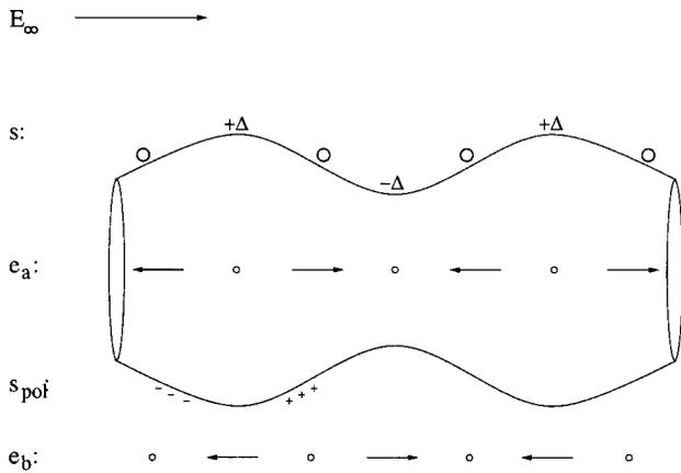
FIG. 9. Physical picture of an unstable perfect dielectric jet; the perturbation in surface charge density causes the electric field perturbation,  $e_a$ ; the polarization charge ( $s_{poi}$ ) tries to cancel out the penetration of the applied field,  $E_\infty$ , and this causes the electric field perturbation,  $e_b$ .
