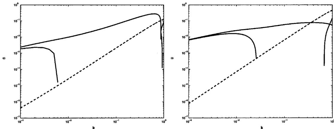
FIG. 20. Comparison of the axisymmetric modes (solid) to the whipping mode (dashed), for the same conditions as Fig. 19, except the jet has a small surface charge  $\sigma_0 = 0.1$ . At low fields, the axisymmetric modes still dominate the whipping mode; however at 5 kV/cm the whipping mode is stronger than both of the axisymmetric modes.
