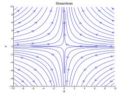
Figure 1: Streamlines plotted in the x - y plane where the arrows are determined by the Eulerian velocity field.
