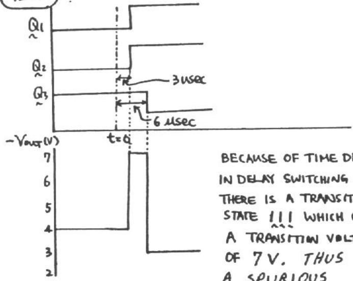
BECAUSE OF TIME DIFFERENCE IN DELAY SWITCHING TIME, THERE IS A TRANSITION STATE !!! WHICH CREATES A TRANSITION VOLTAGE OF 7V. THUS A SPURIOUS 7-V PULSE APPEARS IN THE OUTPUT.
