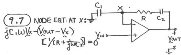
SINCE  $V_{(+)} = V_{(-)} = V_{IN} = V_X$ ,
