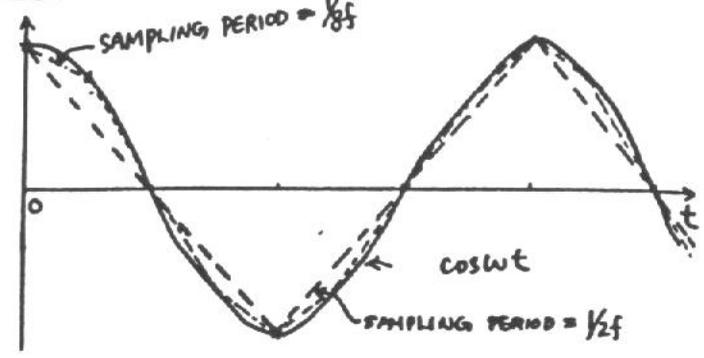
(b) THE GREATEST ERROR OCCURS AT THE PLACE THE CURVATURE (2<sup>ND</sup> DERIVATIVE) IS LARGEST. FOR THE COSINE THIS IS NEAR  $\theta = 0$ . LET THE SAMPLING INTERVAL BE  $\frac{2\pi}{Nf}$ . THE MAX ERROR IS THEN AT THE TIME  $\frac{\pi}{Nf}$ :
