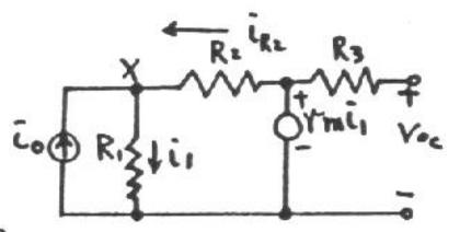
$\bar{i}_o - \bar{i}_1 R_1 + \bar{i}_2 R_2 = 0$
