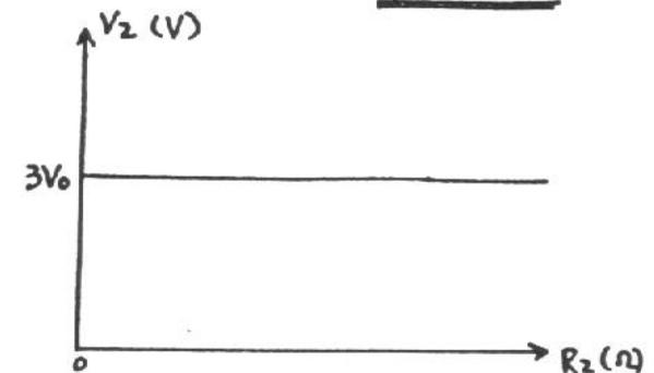
(b)  $i_2 = \frac{\mu V_1}{R_2} = \frac{3V_0}{R_2} A$
