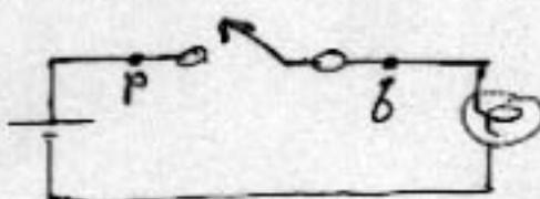
Most direct way of describing the state is by means of a "word statement". There will be a connection between p & q (which implies lamp will be lit) when the switch is closed.
