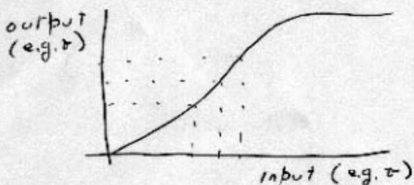
as an analog system each point on the characteristic has equal significance
