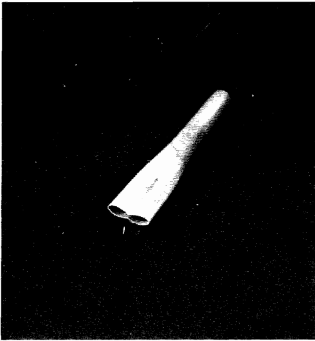
Fig. 5 Section of one of Kyriakides' specimens showing the transition between the buckled and unbuckled regions of the pipe.
