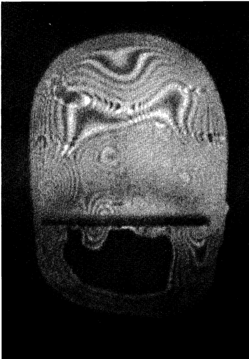
Fig. 14. Decohered region for the relatively thick polyimide film on glass at room temperature.
