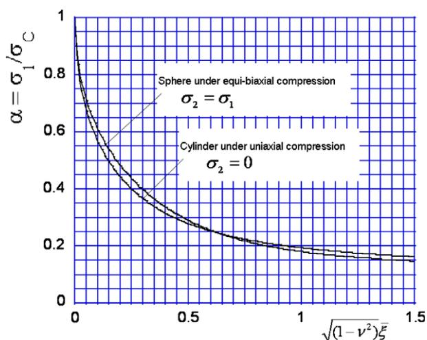
Fig. 3. Imperfection-sensitivity of cylindrical shells under uniaxial compression and spherical shells under external pressure (equi-biaxial compression) based on axisymmetric imperfections (5).
