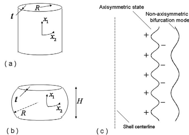
Fig. 2. (a) Cylindrical and (b) spherical shell segments. (c) Interaction between the axisymmetric deformations associated with the initial imperfection and the non-axisymmetric bifurcation mode.
