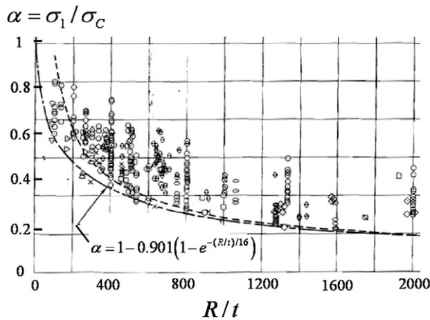
Fig. 1. Experimental data on the knockdown factor plotted against the radius to thickness ratio,  $R/t$ , for cylindrical shells under uniaxial compression. Reproduced from the report of Seide et al. (1960) who assembled the data for shells from various sources. Included in the figure is the empirical NASA (1965) recommendation for the knockdown factor for cylinders under uniaxial compression:  $\alpha = 1 - 0.901(1 - e^{-(R/t)/16})$ .
