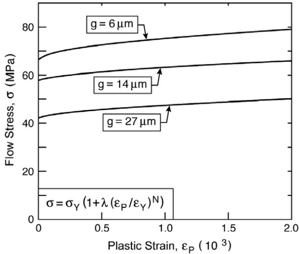
Fig. 2. Tensile stress–plastic strain data for foils with three grain sizes [19–21].
