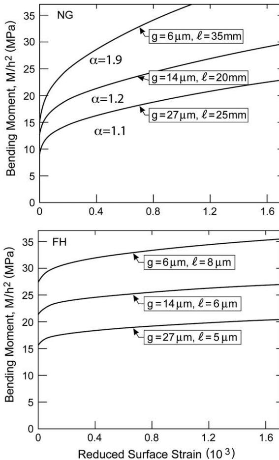
Fig. 6. Predictions of the normalized bending moment  $M/h^2$  as a function of the reduced surface strain for three grain sizes all for foils with thickness  $h = 50 \mu\text{m}$ . In each case, the length parameter was chosen independently to give the best fit to the data in Fig. 1: upper figure, NG theory; lower figure, FH theory.
