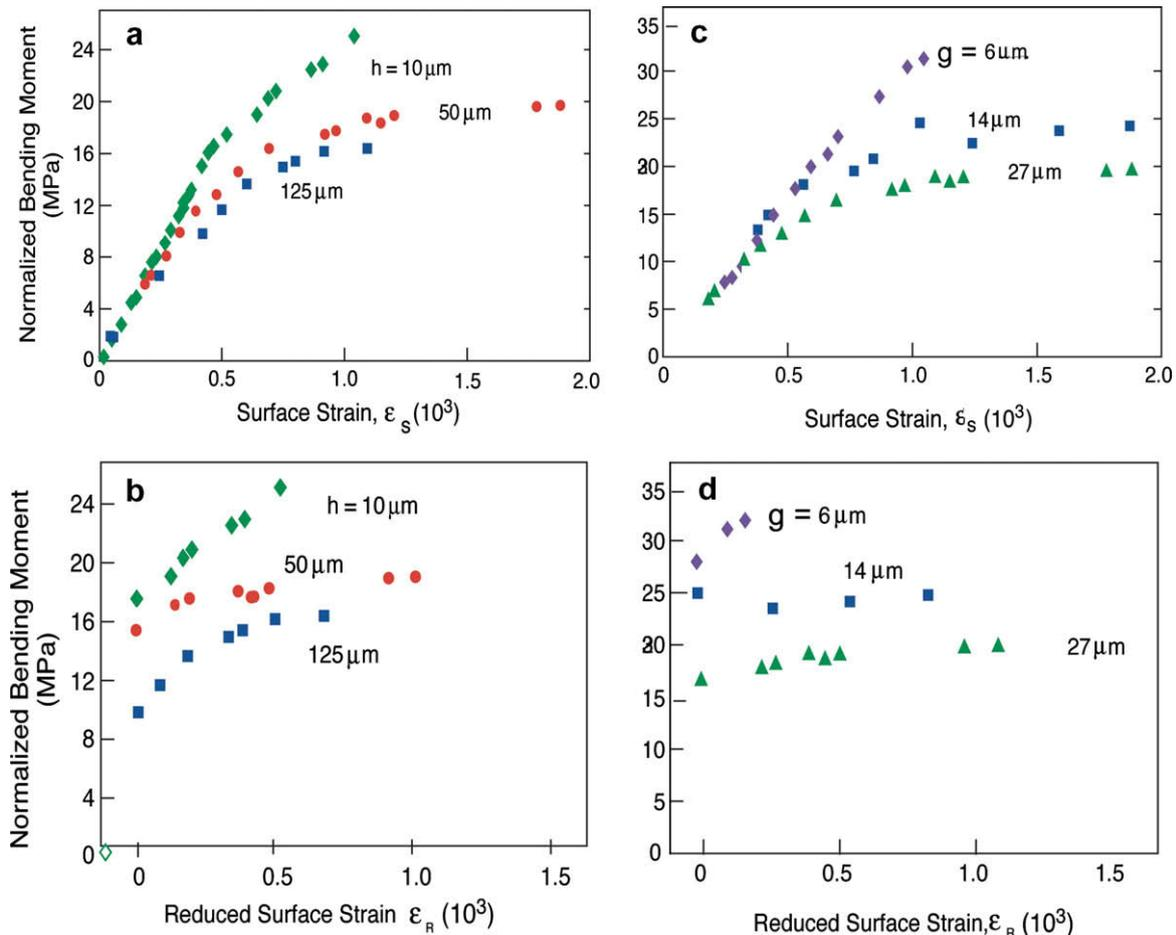
Fig. 1. Normalized moment  $M/h^2$  as a function of surface strain  $\varepsilon_S$  and reduced surface strain  $\varepsilon_R$  for Ni foils: (a and b) for three thicknesses with grain size  $g = 27 \mu\text{m}$ ; (c and d) for three grain sizes with foil thickness  $h = 50 \mu\text{m}$  [19].
