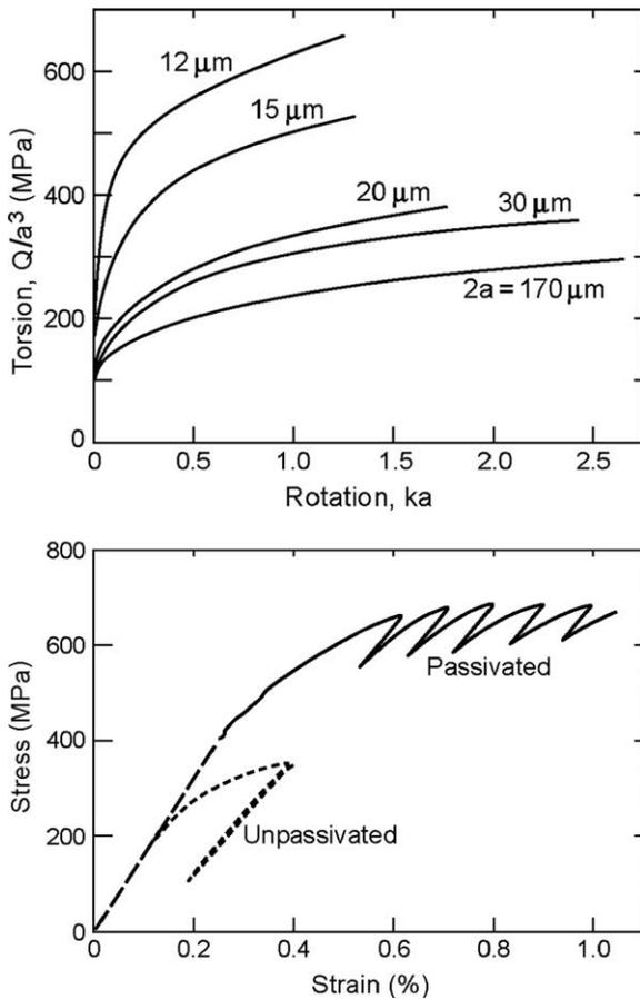
Fig. 3. Upper plot: normalized torque vs normalized rotation for copper wires of various radius  $a$  [7]. This normalization would collapse the data to a single curve if there were no material size dependence. Lower plot: tensile stress–strain data for thin copper films ( $0.34 \mu\text{m}$ ) that are unpassivated and passivated (on one surface) [9].
