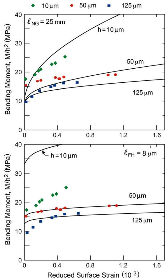
Fig. 7. Comparison between experimental data from Fig. 1 for three foils with grain size  $g = 27 \mu\text{m}$  and theoretical predictions from Fig. 5: upper plot, NG; lower plot, FH.
