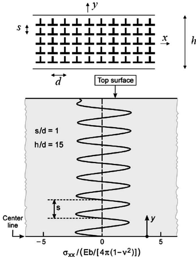
Fig. 14. Horizontal stress distribution halfway between dislocation columns in the upper half of a slab containing a uniform rectangular array of dislocations. The slab is subject to pure bending due to the array with no external loads.
