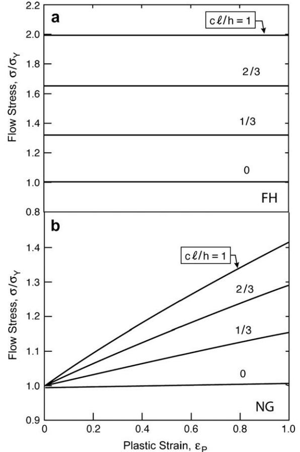
Fig. 4. Trends of average flow stress as a function of average plastic strain  $\varepsilon_P$  for an object of size  $h$  subject to an average gradient of plastic strain  $\varepsilon_P^* = c\varepsilon_P/h$ : (a) FH; (b) NG formulations.
