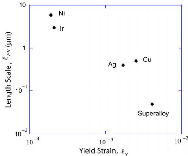
Fig. 13. A plot of the length scale  $l_{FH}$  against the size-independent tensile yield strain. The length scale was ascertained by FH theory using indentation data for Ir [3], a superalloy [30], copper [5] and silver [2], together with the present finding for bending of Ni foils.
