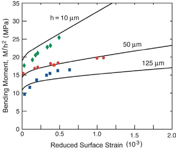
Fig. 12. Prediction from FH theory incorporating a strain-dependent length parameter,  $\ell(\varepsilon_p) = \ell_0(1 + a_0(\varepsilon_p/\varepsilon_Y))$ . The values  $\ell_0 = 2 \mu\text{m}$  and  $a_0 = 0.2$  were chosen both to fit the data for the foil with  $h = 50 \mu\text{m}$  at  $\varepsilon_R = 10^{-3}$  and to represent better the initial increase in strength and hardening of the foil with  $h = 10 \mu\text{m}$ .
