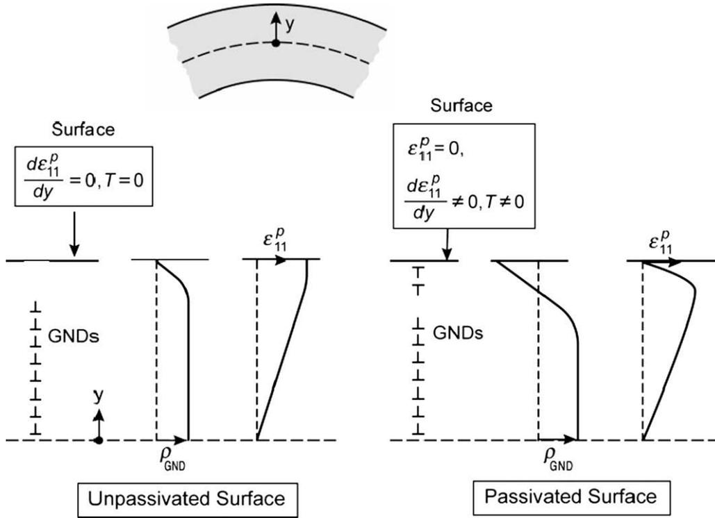
Fig. 11. Schematic of dislocation and plastic strain distributions in bending for foils with unpassivated and passivated surfaces.
