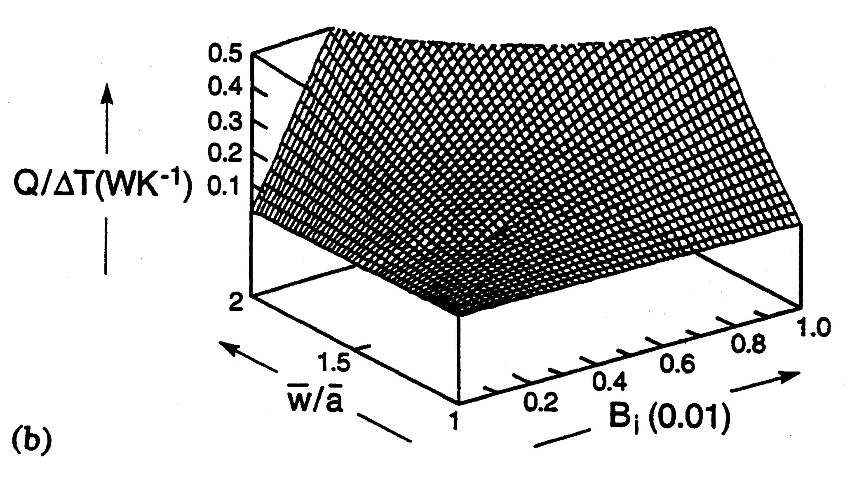
Fig. 12 (a) Power levels achieved with perimeter cooling, as functions of the Biot number and chip density (a/b = 5, w/a = 2, and k = 500 W/mK); (b) the effect of enhanced cooling on the power levels for perimeter cooling  $(a/b = 5, w/a = 2, \bar{a}/w = 10, \text{ and } k = 500 \text{ W/mK})$ .
