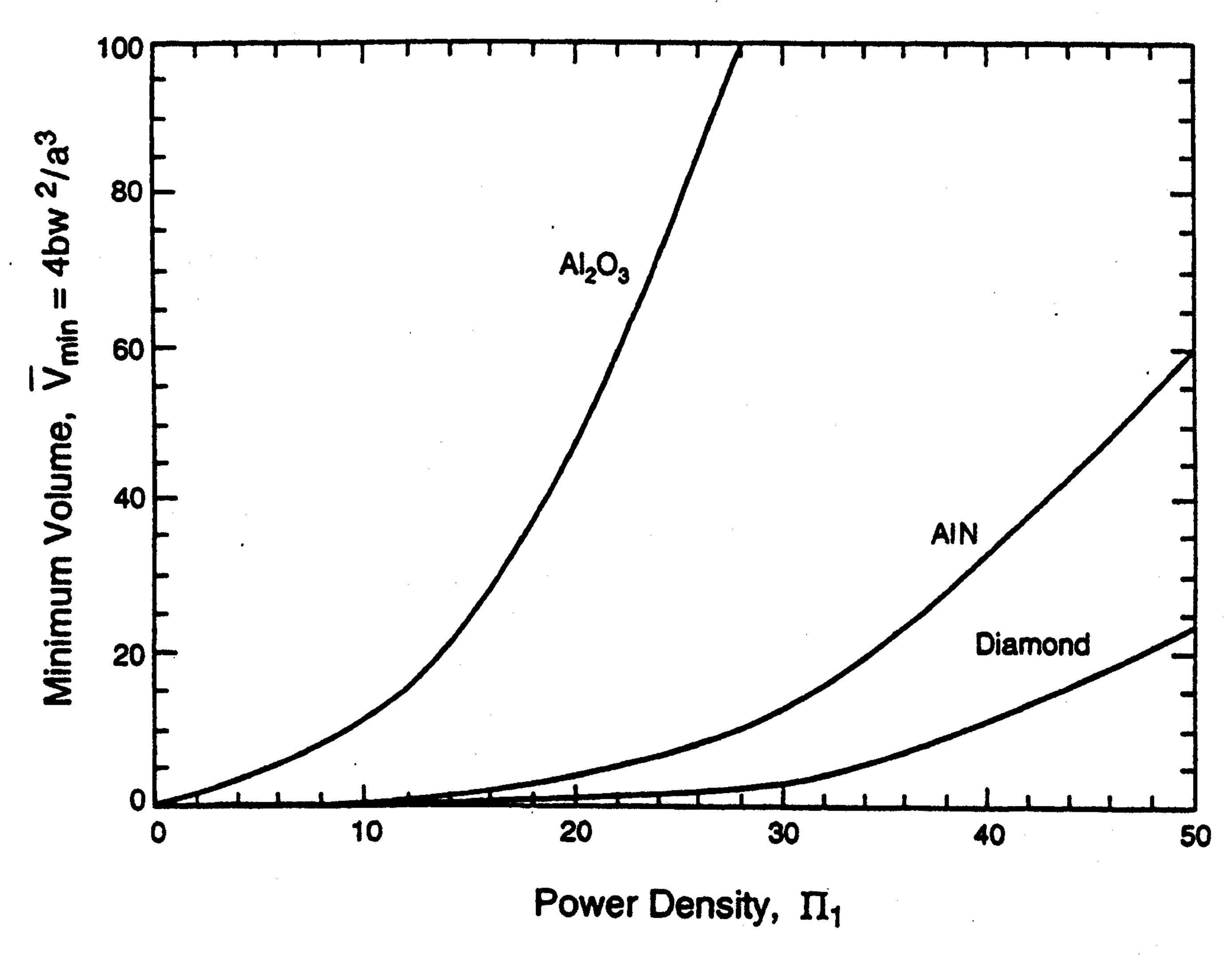
Fig. 9 Nondimensional minimum substrate volume  $V_{min}/a^3$  as a function of power density,  $\Pi_1$ , for  $Al_2O_3$  ( $B_i = 10^{-2}$ ), AlN ( $B_i = 8 \times 10^{-4}$ ), and diamond ( $B_i = 10^{-4}$ ).
