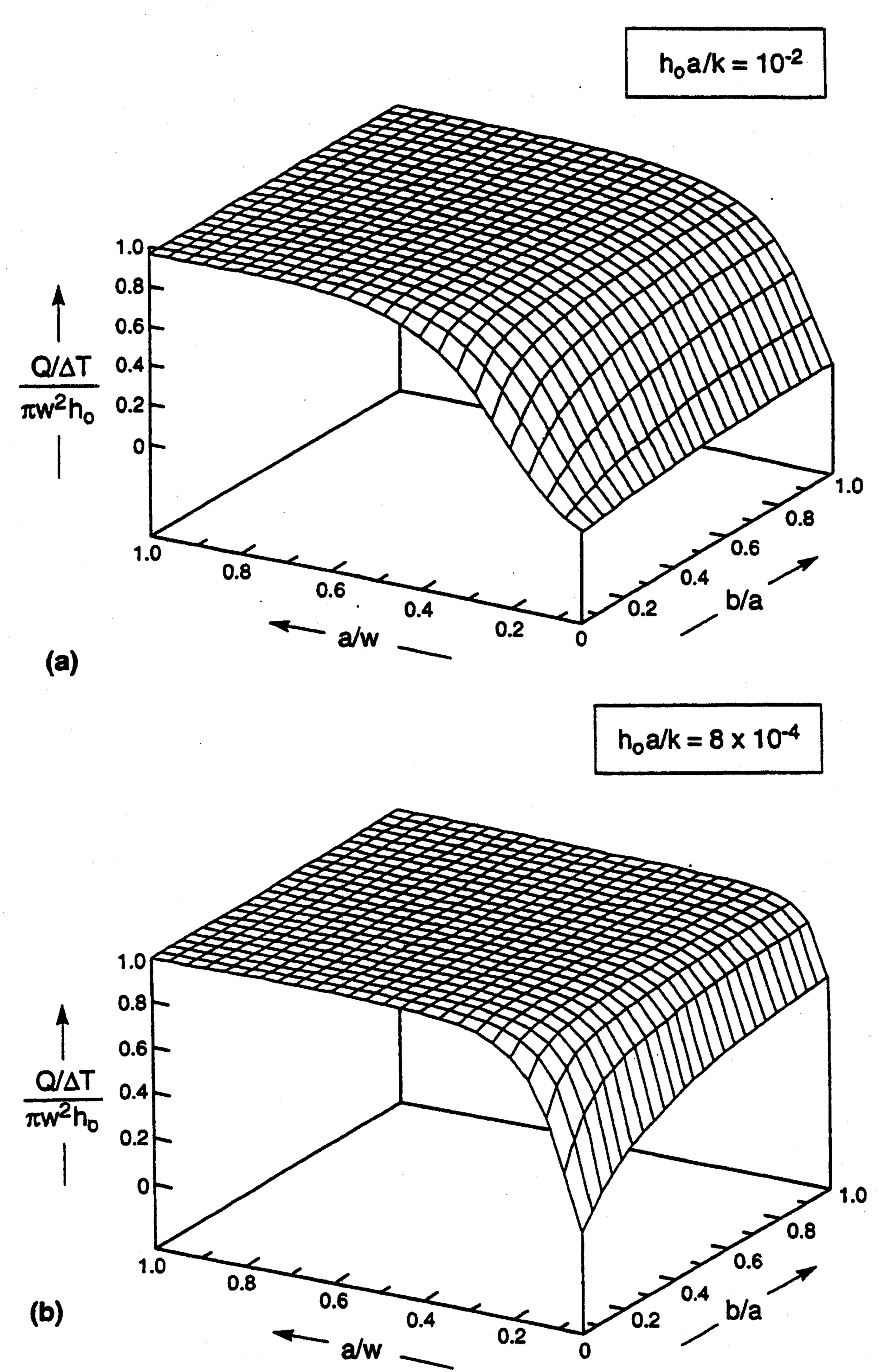
Fig. 10 The effect of substrate dimensions on the overall power density,  $\Pi_2$ : (a)  $B_i = 10^{-2}$  and (b)  $B_i = 8 \times 10^{-4}$ .
