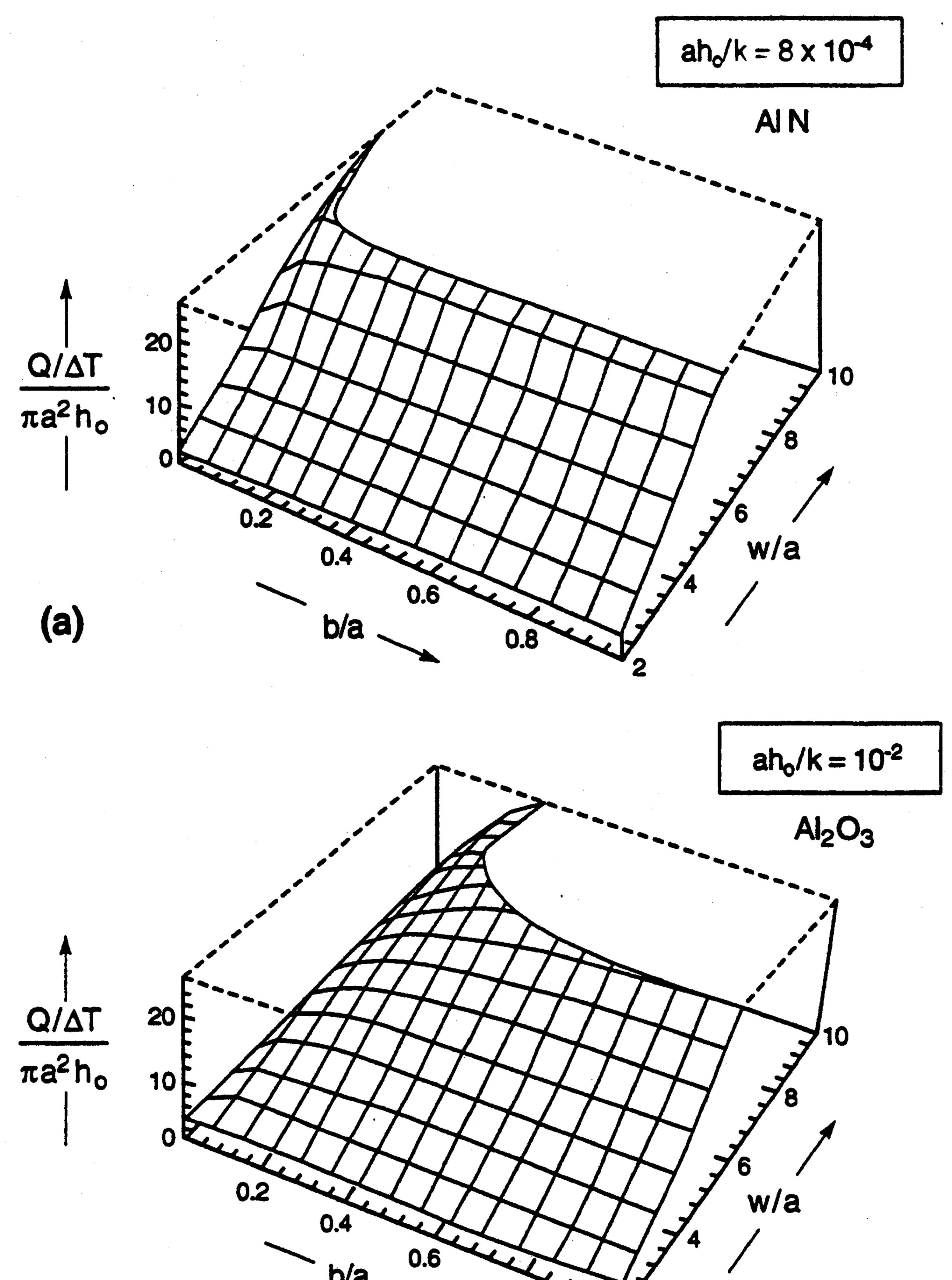
Fig. 8 Power density maps at relatively high chip densities indicating the range of substrate dimensions needed to achieve a power level,  $\Pi_1 = 25$ : (a)  $B_i = 8 \times 10^{-4}$  (AIN) and (b)  $B_i = 10^{-2}$  (Al<sub>2</sub>O<sub>3</sub>).
