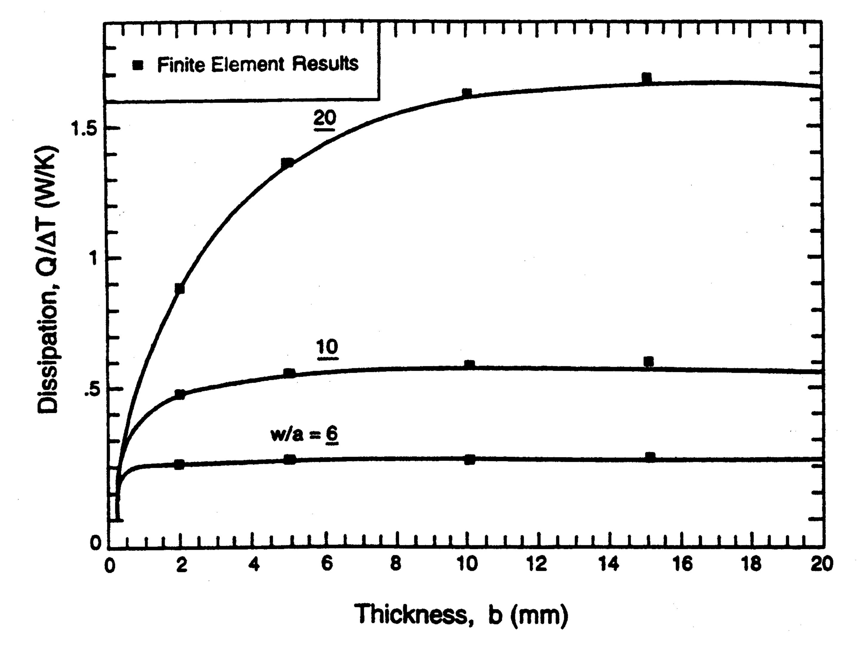
Fig. 4 Variations in power with substrate dimensions comparing magnitudes calculated using the shear lag model with those determined using finite elements. Similar levels of agreement are found over the full range of parameter space explored in this study.
