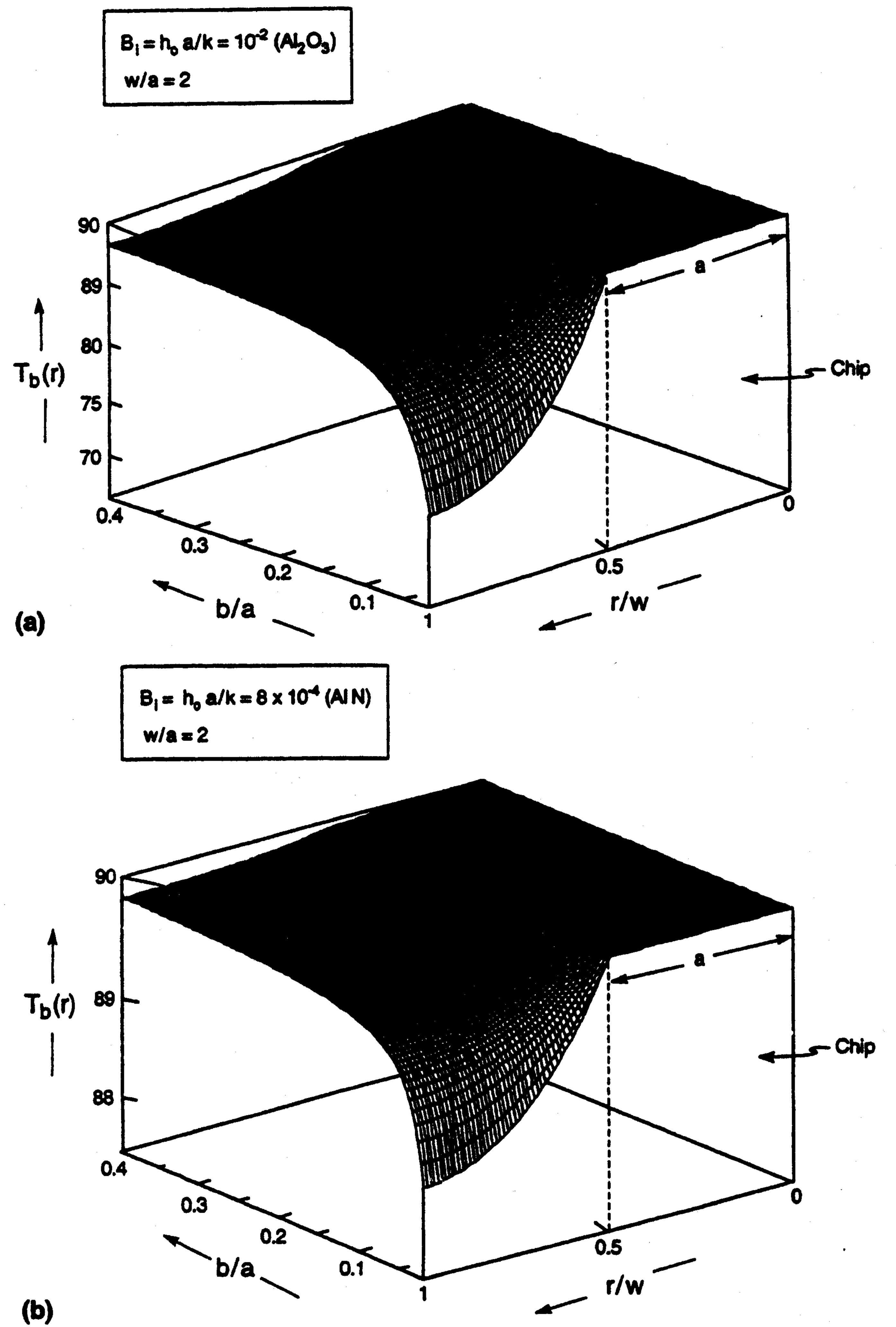
Fig. 5 Temperature distributions on the lower substrate surface indicating the role of substrate thickness, b/a for a chip density a/w = 0.5. Results are presented for two Biot numbers: (a)  $B_i = 10^{-2}$  representative of  $Al_2O_3$  and (b)  $B_i = 8 \times 10^{-4}$  representing AIN.
