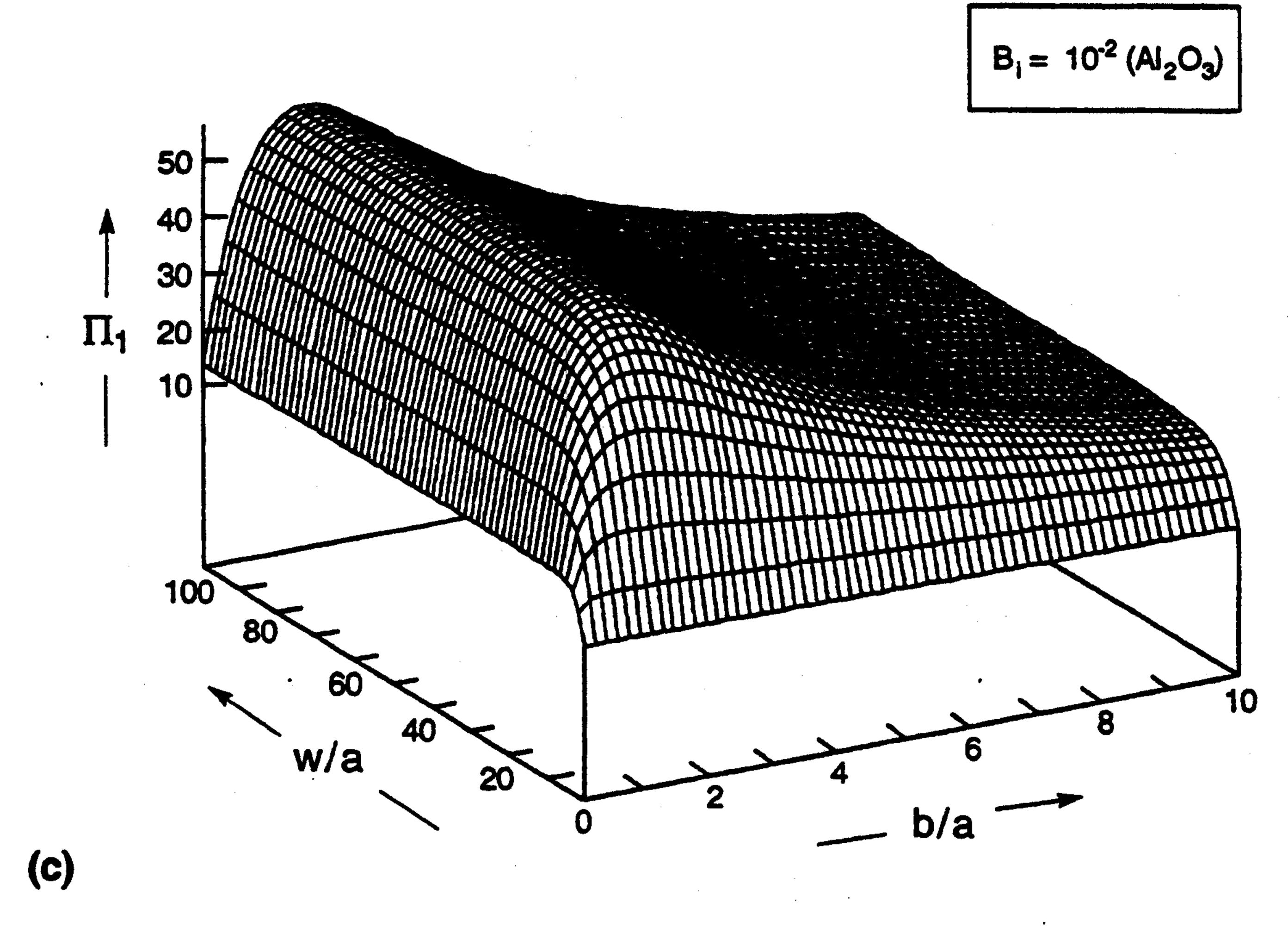
Fig. 7 Power density maps illustrating effects of chip density and substrate thickness at three levels of Biot number: (a)  $B_i = 10^{-4}$  (diamond), (b)  $B_i = 10^{-2}$  (Al<sub>2</sub>O<sub>3</sub>), and (c)  $B_i = 8 \times 10^{-4}$  (AlN).
