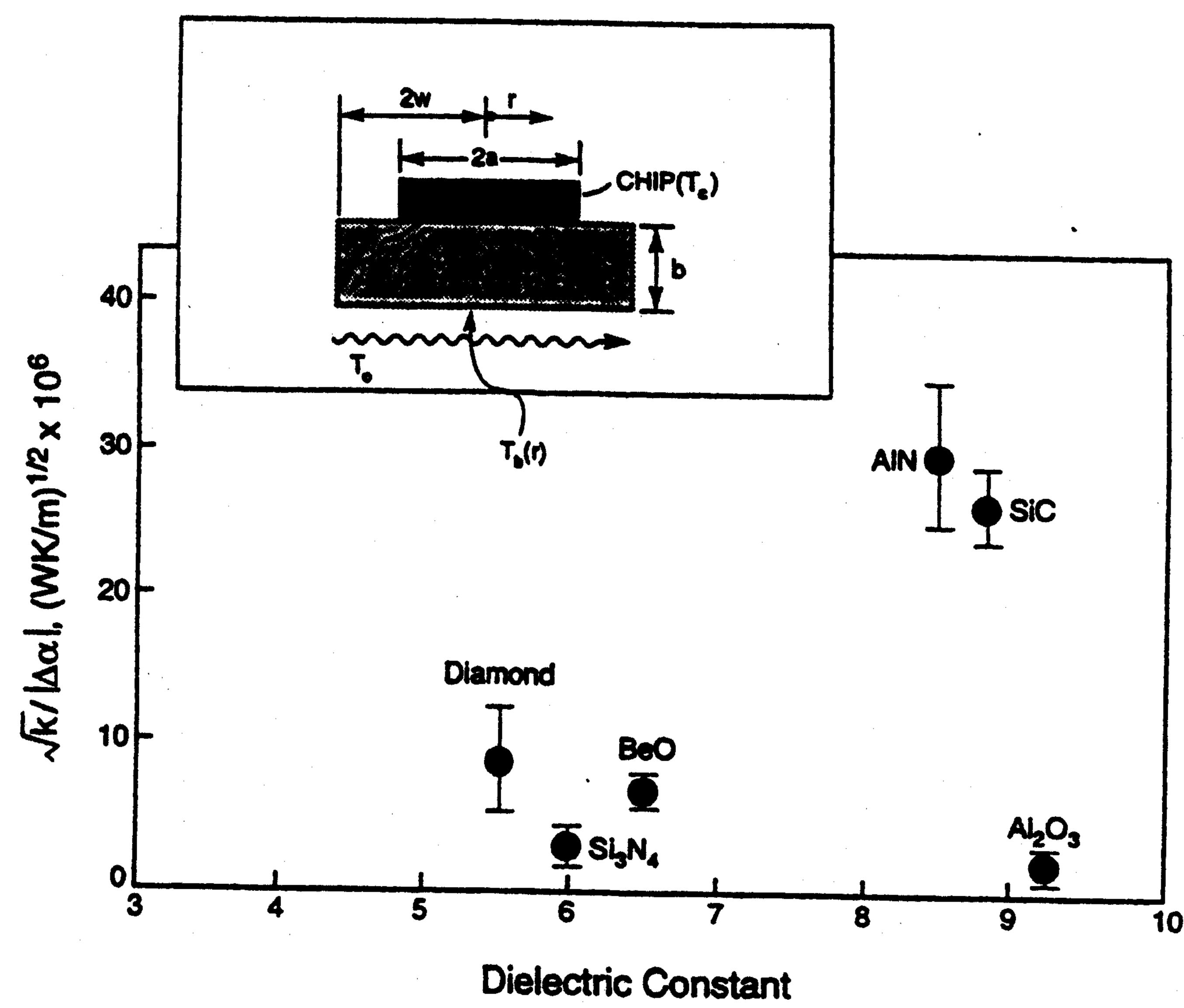
Fig. 2 A material selection diagram for high heat dissipation substrates. Large values of the ordinate and small value of the dielectric constant constitute the preferred materials. The insert shows the configuration that determines the material selection index.
