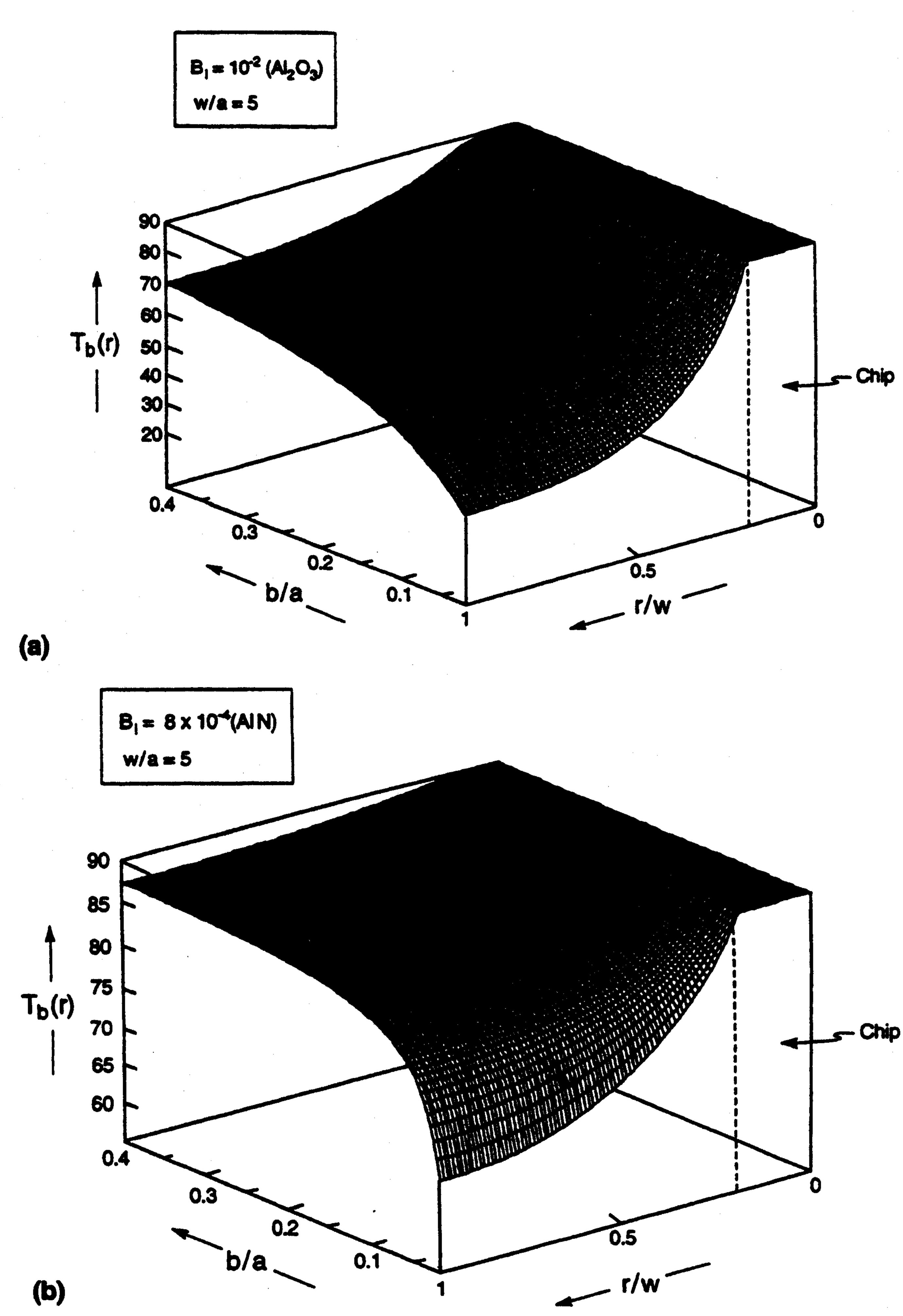
Fig. 6 Temperature distributions for a chip density, a/w = 0.2: (a)  $B_i = 10^{-2}$  (Al<sub>2</sub>O<sub>3</sub>) and (b)  $B_i = 8 \times 10^{-4}$  (AlN).
