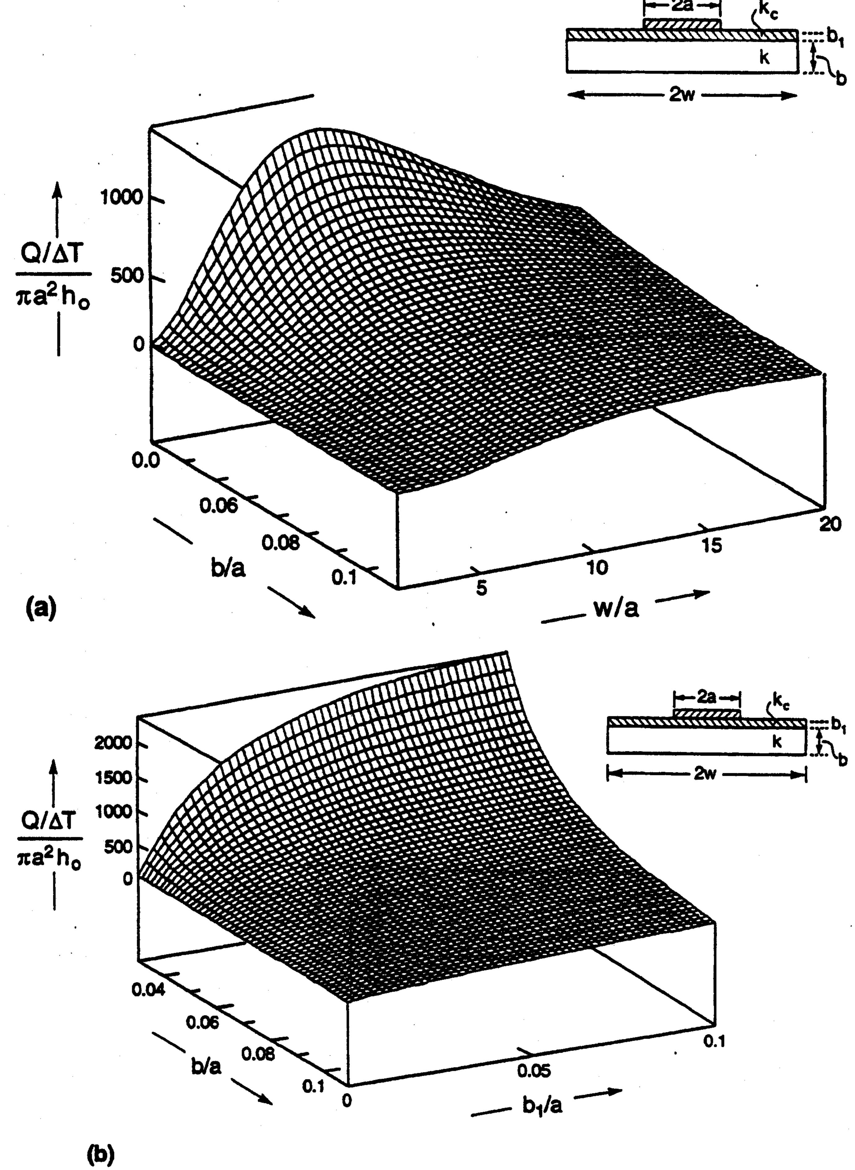
Fig. 11 The effect of a highly conducting layer on the power density,  $\Pi_1$ : (a) trend with substrate dimensions and (b) the influence of layer thickness,  $b_1$ . These results have been obtained by using the properties of AIN for the substrate and diamond for the layer.
