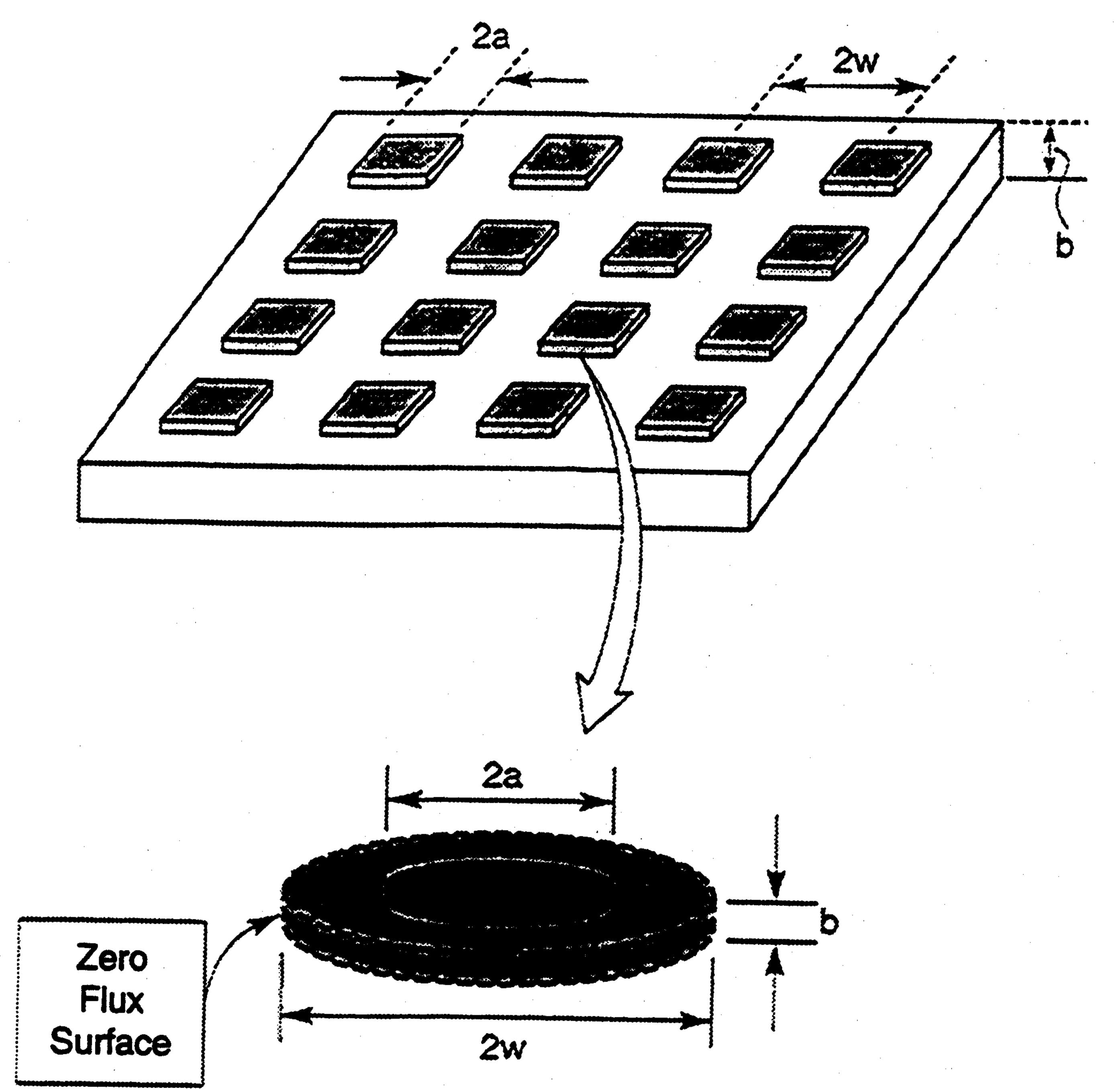
Fig. 1 Prototypical multichip module design cooled from below by forced convection. The representative cell is shown.
