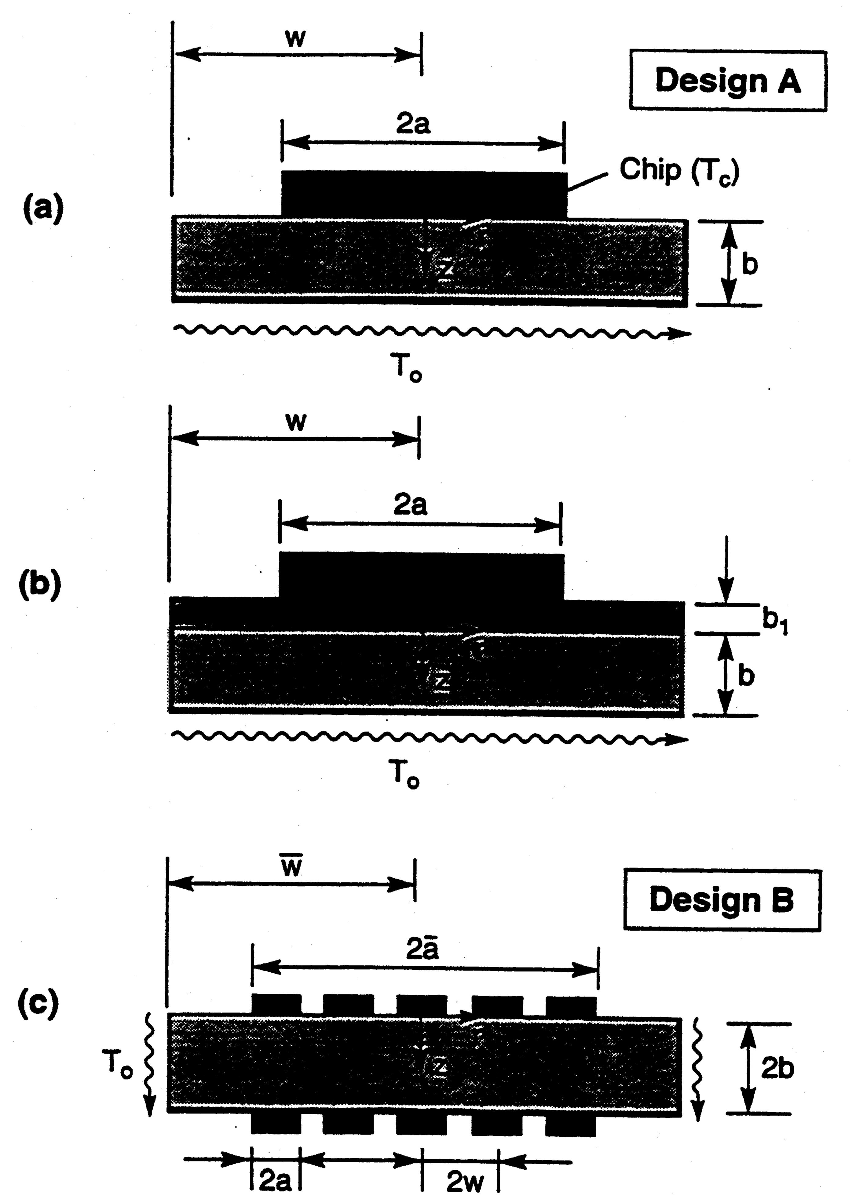
Fig. 3 Multichip module designs considered in the present analysis: (a) representative unit cell for a Monomaterial substrate with convective cooling from the lower surface, (b) bimaterial substrate with convection cooling, and (c) compact multichip module with perimeter cooling.
